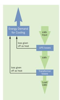
In data centers losses incurred by inefficient distribution transformers are amplified by the inefficiency of the UPS. Furthermore, as all losses are given off as heat, energy losses incurred by transformers and the UPS increase the cooling demand.
