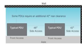
Typical PDU Footprint (per NEC)
