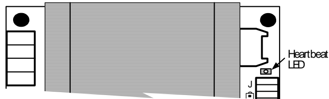
Figure 6-3: Location of Heartbeat Light on Power Monitor (Cyberhawk-PMP 30)
